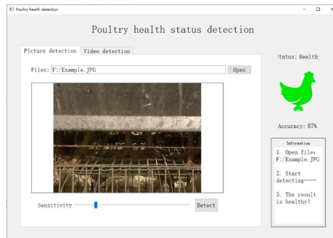
Figure 12. The software interface implemented by the disease detection function; by detecting the visual part of the poultry (the standing area below the feed trough), the current behavioral state of the poultry (standing, lying on the stomach) can be judged, and the health state of the chicken can be inferred.
